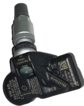
Figure 1.1: TPMS smart valve
