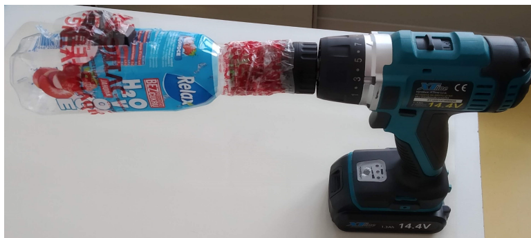
Figure 3.8: Rotational velocity measurements on a valve attached to a drill
