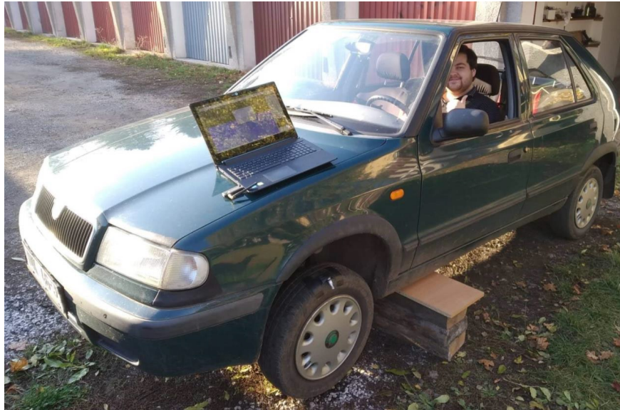
Figure 3.9: Rotational velocity measurements on a valve externally attached to a wheel of a car
