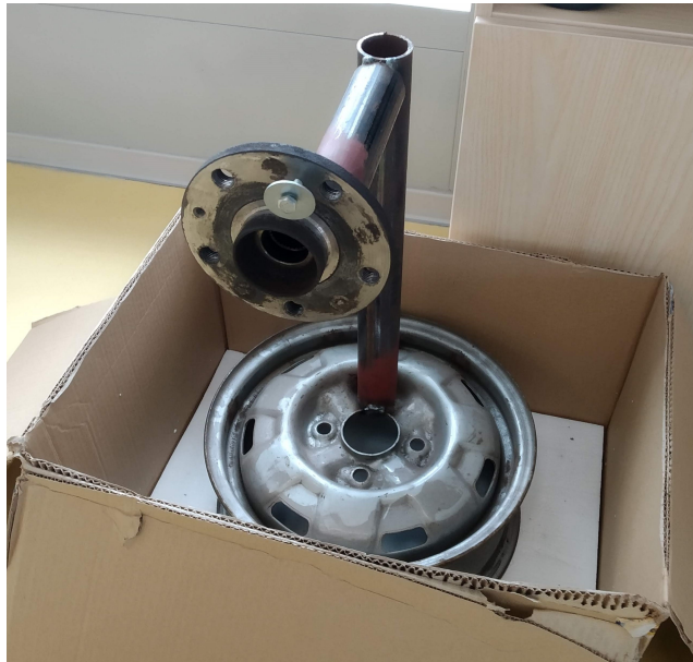
Figure 3.3: Welded wheel holder with a rotatable plate
