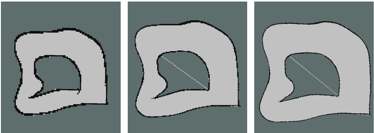
Figure 3.5: Maps of the track with different resolution (0.1m, 0.05m, 0.025m)
